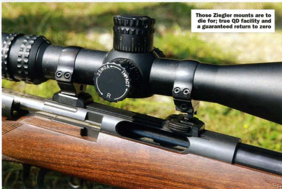
The barrel is well free-floated, which must contribute to the Lynx's accuracy potential
