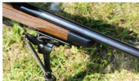
The barrel is well free-floated, which must contribute to the Lynx's accuracy potential
